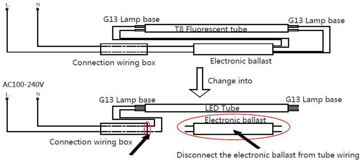
Please connect the wiring according to diagram and connect the wiring per diagram in the wiring box
